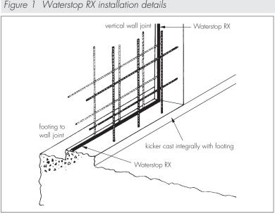
Figure 1 Waterstop RX installation details
